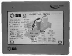
Vision 2020i, an advance programmable electronic controller designed specifically for the applications and precise control of Dunham-Bush Variable Speed Rotary Screw compressor chillers, WCFX-V.
