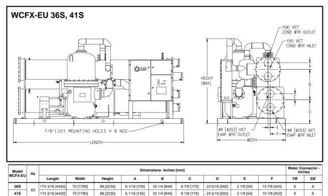
Notes: 1.) Above drawings and dimensions are models with vessels construction based on flat head and comply with PED/ Chinese Machinery codes. 2.) Unit layout shown are for reference only. Some orientations may vary.
