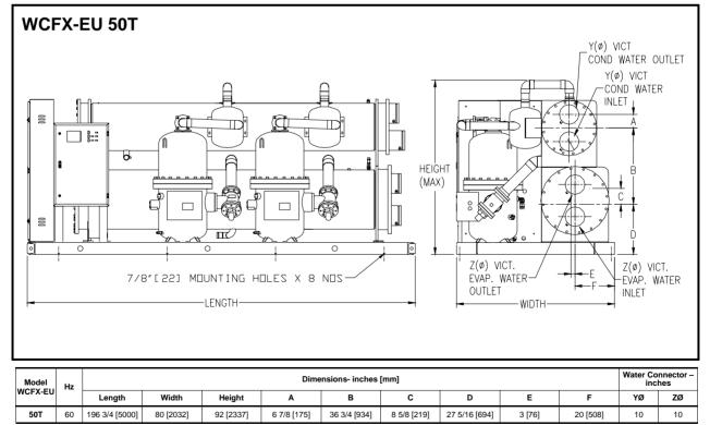
Notes: 1.) Above drawings and dimensions are models with vessels construction based on flat head and comply with PED/ Chinese Machinery codes. 2.) Unit layout shown are for reference only. Some orientations may vary. 3.) Consult factory for models with ASME/ other approved vessels.
