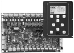
DB-Director is a rugged microprocessor based controller designed for the HVAC/R applications. DB-Director provides flexibility with set points and control options that can be selected prior to commissioning a system or when the unit is live and functioning. Displays, alarms and other interfaces are accomplished in a clear and simple language that informs the user the status of the chiller.
