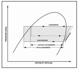
Liquid refrigerant enters the flooded evaporator uniformly where it absorbs heat from water flowing through the evaporator tubes, and vaporized. The vaporized refrigerant is drawn into the compressor suction port where the positive displacement compression begins.
