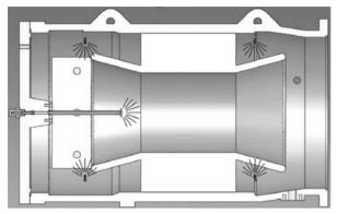
The DCLCD compressor motor is cooled by an efficient refrigerant spray cooling system. Refrigerant spray cooling method is more efficient than other methods.
