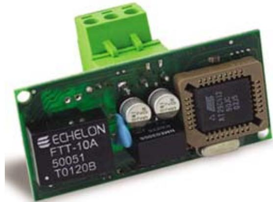
The LONWORKS Card is the protocol that was Created by Echelon Corp. The LONWORKS is a leading networking solution for building automation. The communication is based on the FTT10 electrical standard.
